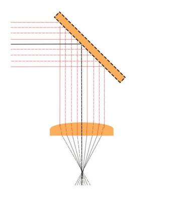
**Step 16: Incorrect Vertical Beam Alignment**
