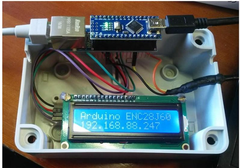
This version has the quickest and easiest assembly of all. One needs to file holes for cables and to glue LCD. That's it. But in order to change Eth cable or USB cable one needs to unscrew the box lid which is an easy work. Nice dust protection.
