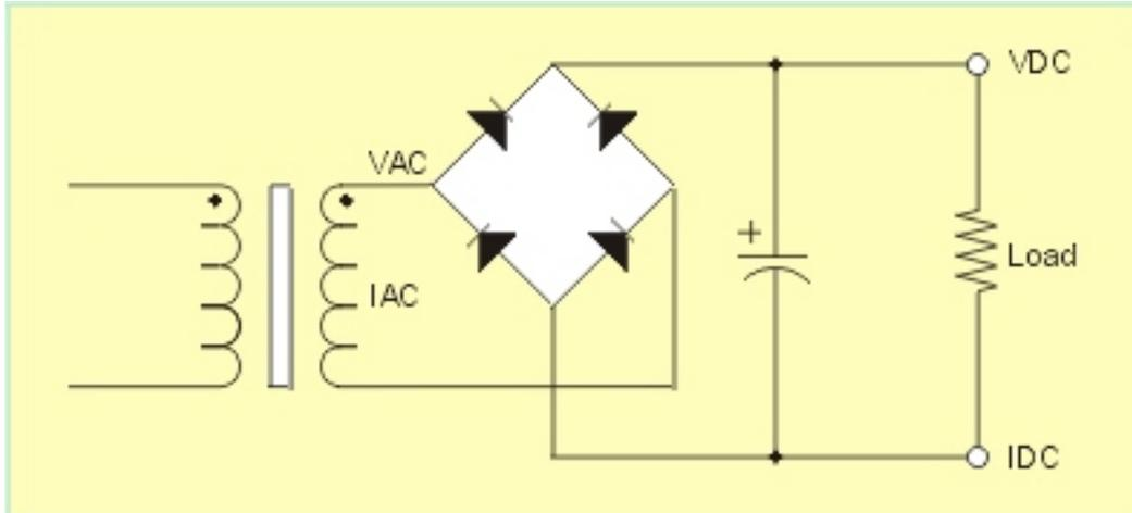
The picture above shows the proper connection from the secondary of the transformer to the bridge rectifier and the connection from the bridge rectifier to the filter capacitor.
