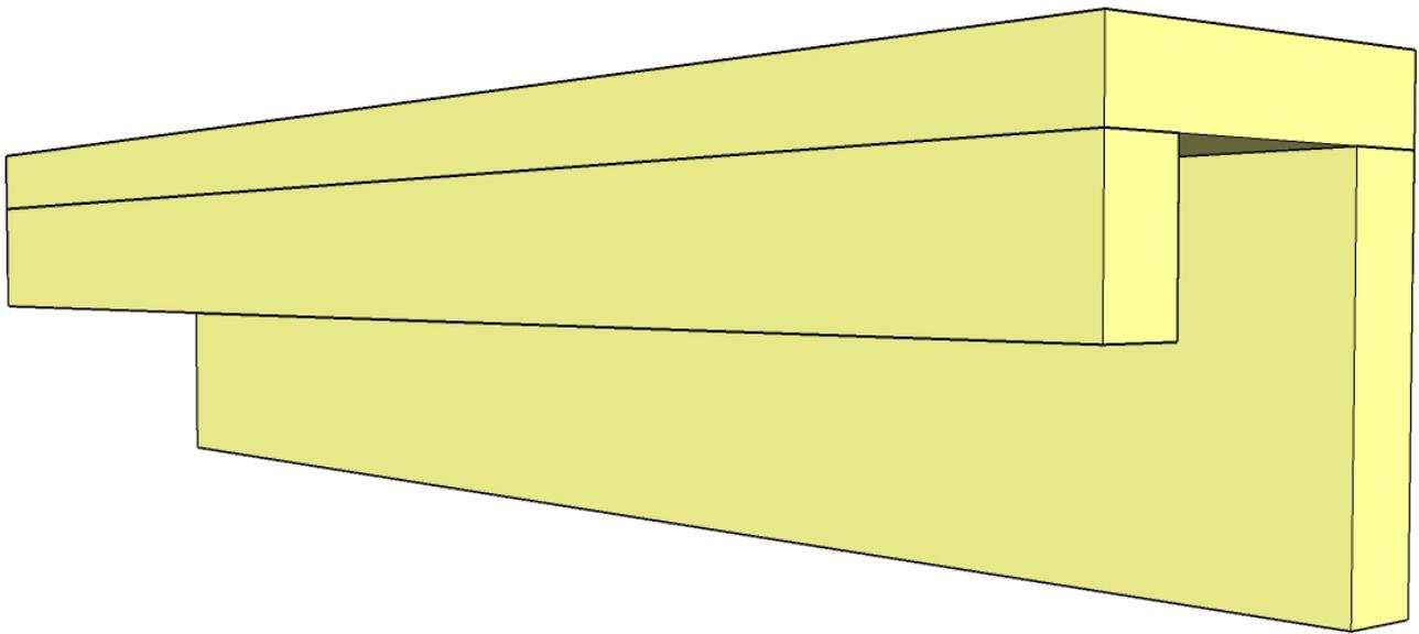
The only trick to watch with the Guide Box is **NOT** to add glue to the front face as you will need to remove it to screw the cleat to the wall. Space your pocket holes to give you room to drill the mounting holes in between.
