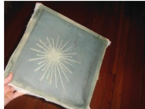
**Figure K:** Rinse the screen carefully
