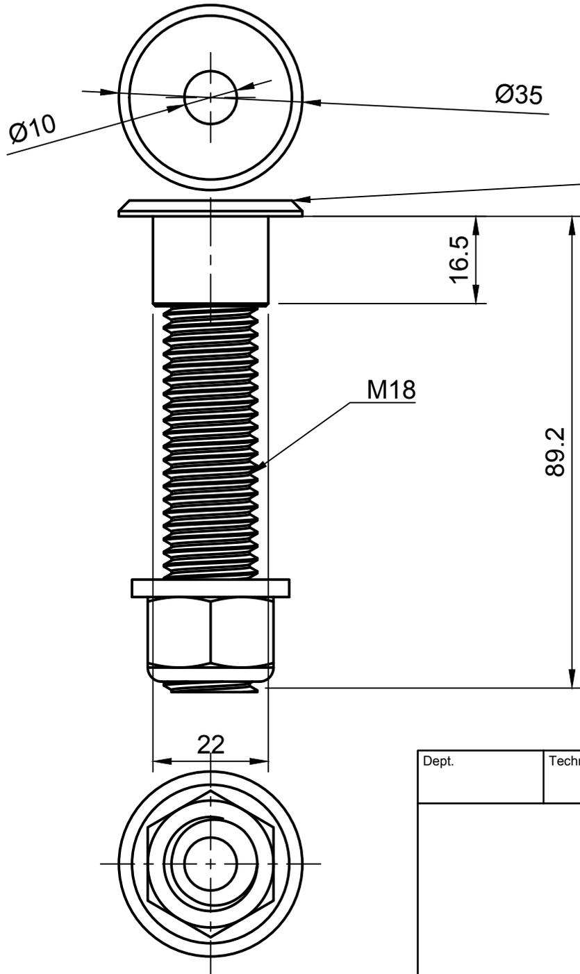
ANGLE NOT CRITICAL, SMALL DIAMETER MUST BE 20
