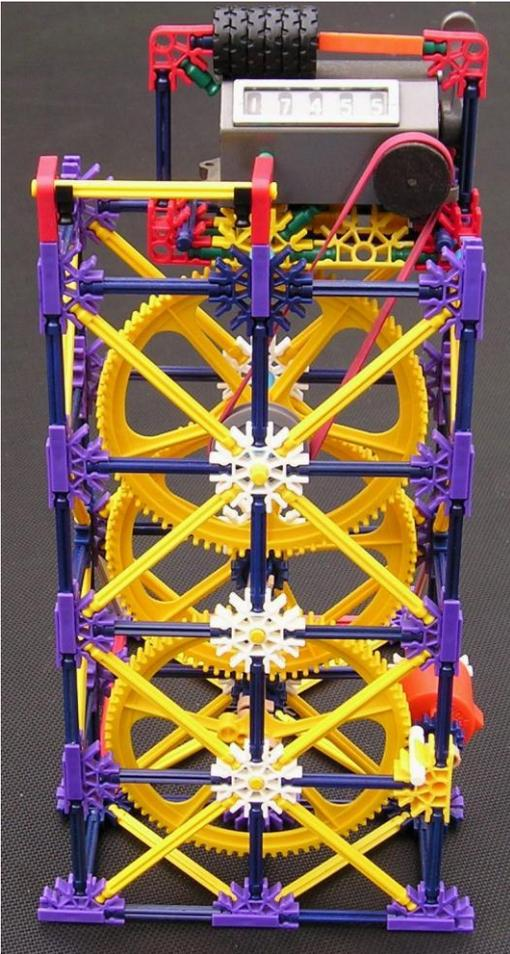
On the left is a solar-powered K'Nex counting machine (the counter at the top was made by English Numbering Machines and is not a K'Nex component). The small black wheels at the top simply help to hold the counter in place. In bright sunshine, the counter is incremented by 1 about every 5 seconds.
