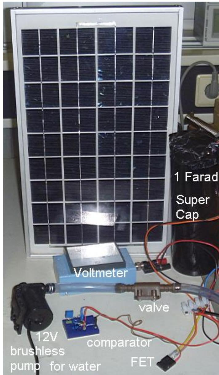
Solar pump can be used to pump water for irrigation of a greenhouse. It happens often that that the day is cloudy and the current from a solar panel drops to ca 10 % of peak, that is no longer enough to drive a motor. Solution would be to have an overdimensioned panel (100 W to drive 10 W pump).
