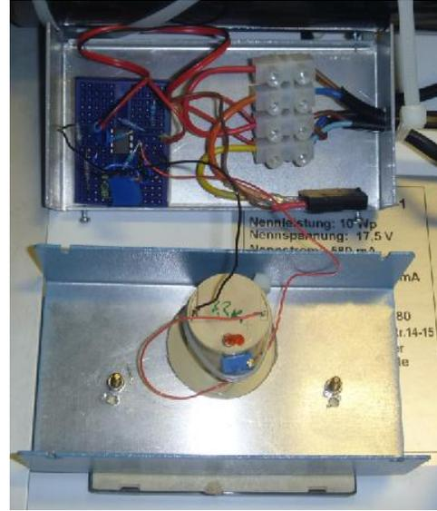
Test construction was done on a solderless breadboard and later fitted into outdoors-qualified enclosure.
