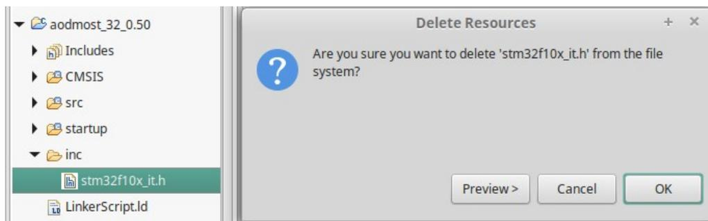
Now you can import AODMoST 32 files into aodmost\_32\_0.50 project. Copy init.c, main.c (overwrite previous file), sbs.c and tb.c into src folder. Copy config.h, init.h, main\_functions.h, main\_variables.h, sbs.h and tb.h into inc folder. When you are done it should look like this:
