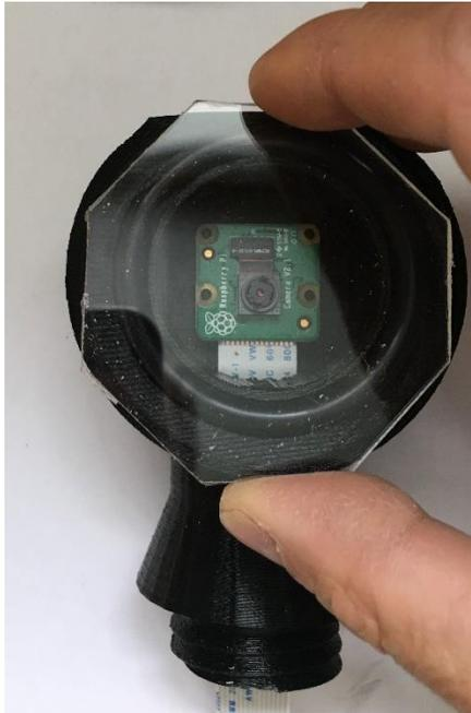
5. Screw the 89 mm locking collar securely over the plexiglass window in the direction shown until some resistance is felt. **DO NOT OVER-TIGHTEN!**
