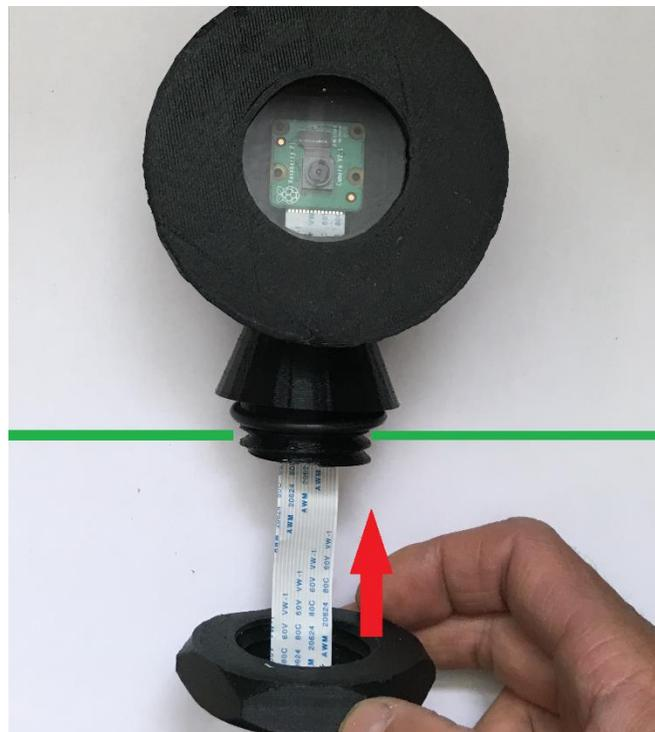
9. Connect the free end of the ribbon cable onto your other equipment (ex: Raspberry Pi computer board) and test it out. If the Raspberry Pi camera board is not suitably level within the WeatherBox, the rim of the WeatherBox might be visible in your pictures. Unscrew and remove the plexiglass plate and O-ring, and use the erasure from a pencil or similar device to gently poke down the corners of the circuit board.
