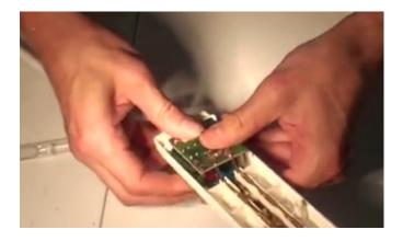
Replace the screws and collar that held the input power cord into place.
