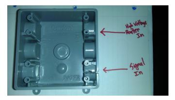
Insert and screw in the NM/SEU cable connectors into the port marked "high voltage router".
