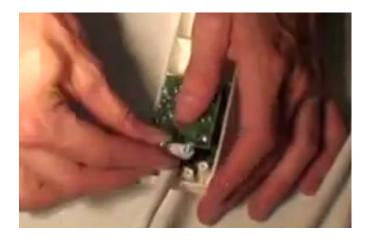
Pull out the input power cord and remove the guts of the power strip.
