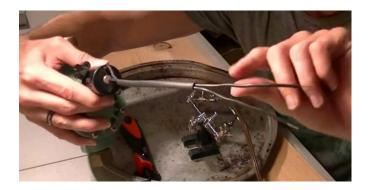
Now solder the two wires together but do not heat seal the shrink wrap yet.
