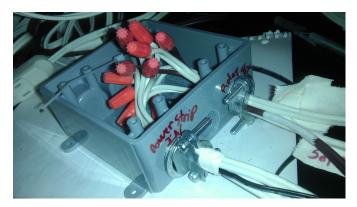
Now to test the high voltage router, you must temporally cap off each of the four cable pairs coming out that will go to the relay shield from the port labeled "relay out". This will simulate all of the relays being turned on and closing their corresponding circuits. Again this allows all electricity to flow through the circuit and this needs to be done on a clean non-electrically conductive table with hand and tools away from the high voltage router.
