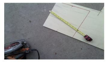
Draw the template onto the cut board.
