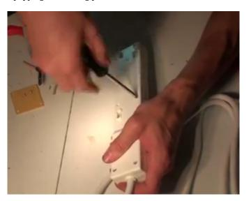
Remove the screws and collar that hold the input power cord in place
