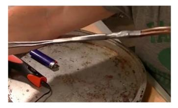
This is what you should end up with. These are ready to plug into the female extension cords that will come out of the bottom of the control unit.
