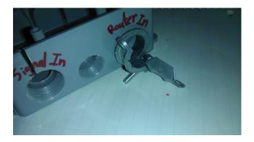
Route the high voltage relay lines from the high voltage router through the appropriate port on the relay shield breaker box. Do not tighten down the cable connector clamp on the relay shield breaker box until the relay lines are later secured in a relay terminal.
