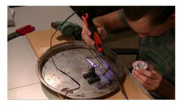
Once you are done with the soldering, you'll have to insulate the two wires from each other with two simple wraps of electrical tape. Just make sure that there is no exposed metal from the solder job that could potentially arc out or short from wire to wire.
