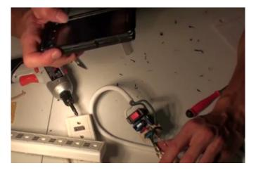
With a heated soldering iron, remove the soldered leads that connect the power cord to the power strips internal circuitry.
