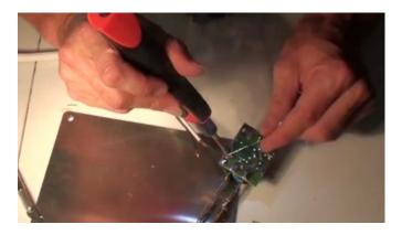
Replace the guts into the power strip frame.
