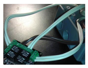
Then, lightly pull the wire pairs back through the breaker box port until a comfortable amount of wire is left inside the relay breaker box. Then tighten down the cable connector clamp to keep the wires in place inside the relay shield breaker box.
