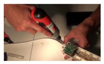
Replace the back and screw in the backing screws to the power strip.
