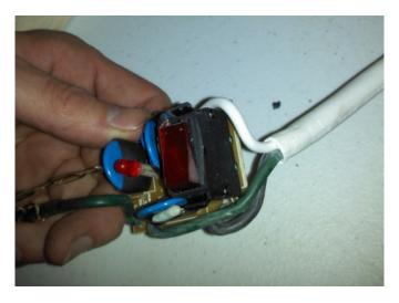
Make sure to take a picture of all angles of the soldiered connections inside the power strip so that you can solder new connections appropriately for your model of power strip. This is important and confusion here will produce shorts and potentially dangerous results.
