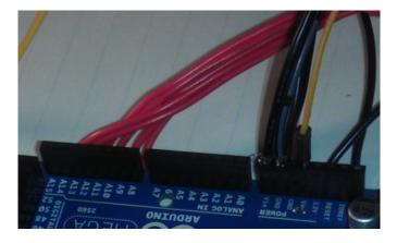
Begin by heating up your soldering iron and soldering the 7 sensor signal wires to the bottom of the Arduino. The pins that this project uses are analog output pins. The 2 for the temperature sensors are A8 and A9. The pins for the moisture sensors are pins A11, A12, A13, A14, and A15. Don't hold the soldering iron to the metal for more than three or four seconds without pulling it away and letting the board cool. It's pretty easy to burn a PCB board like an Arduino.
