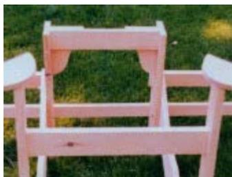
**5** - Cut part **S4** to **2 5/8" x 17"** (6.7cm x 43.2cm), and clamp centered between back supports E, 20" from the ground, like the outer arms, parts G. Attach with 2 screws in each end, through parts E.
