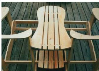
**8** - Using an adjustable square, or plum line, line up the lower slats with the upper slats, and screw in place with one screw into the front and back joiner strips. The back curve should line up with the upper shelf curve, but the front lower shelf does sit out further than the upper shelf.
