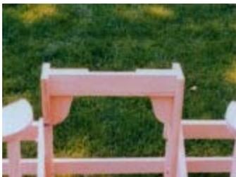
**4** - Cut part **S3** to **2 5/8" x 13 3/4"** (6.7cm x 34.9cm), and clamp behind arm supports F, flush with the tops. Attach with 2 screws in each end, through parts D, the arm supports.
