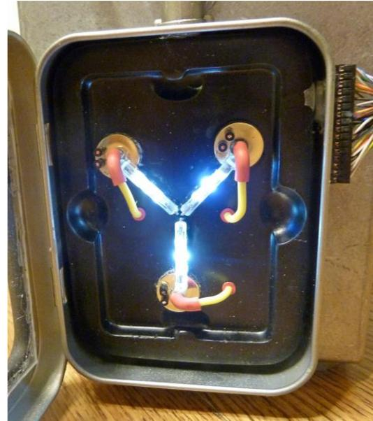
The "vacuum tubes" started out as real vacuum tubes. Wrap the tubes in a paper towel then gently break the glass. It doesn't take much. Using the insides, an LED will fit up inside. The bases are those LED tea lights from the dollar store, painted black. The "glass" parts are cut down plastic candy tubes from eBay.
