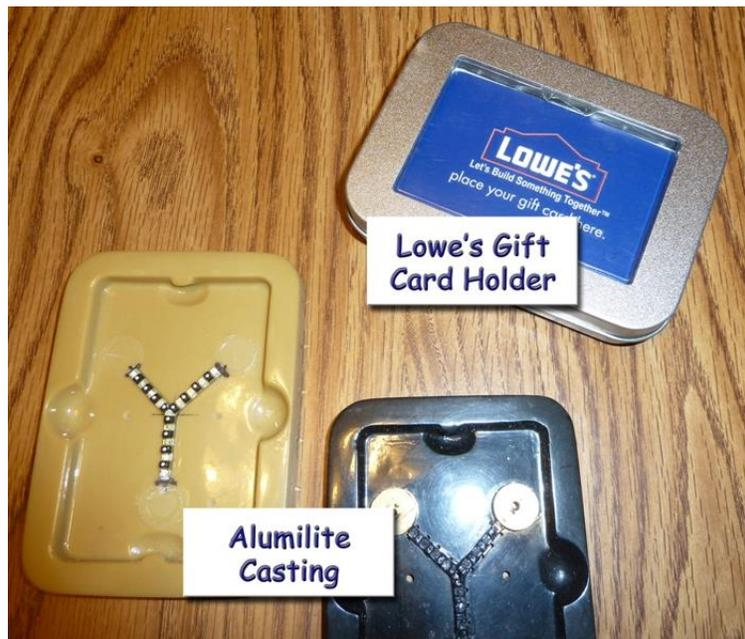
I removed the card holder insert, made a mold, and poured a solid version, using Alumilite. I got some of those flashy pins from Party City for the electronics. Xenon Strobe Flash Tubes from eBay & some brass snaps from Hobby Lobby, for the vacuum relays. The tiny LEDs come from eBay. For the wires, I used I
