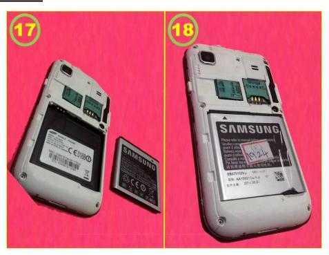
Take the phone and remove the battery and wait for a minute. Then Insert the batter to your mobile and do not press any buttons.
