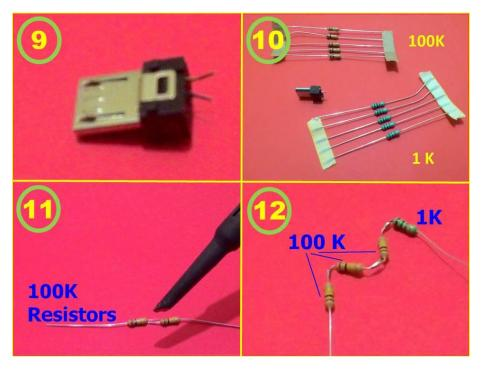
The Pins are so tiny. So, insert two thin pins in the chamber of Pin No. 4, 5 tightly alongwith the exiting one, so we can easily solder the resistors (Fig.(9)). The JIG may works fine from 300K to 400K, typical value is 301K. Solder three 100K Resistors and one 1K Resistors one by one (Fig.(10) &(11)). Bend the Resistors as shown in picture as shown in Fig.(12) so we can house in the case.
