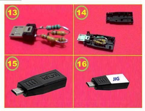
Solder the resistor series between Pin No. 4 & 5 of MicroUSB Pin as shown in Fig (13), Place them in the case (Fig.(14)) close it tightly Fig.(15)). Wrap it with sticker and write any marks (Fig.(16) to avoid miss handling by some others. Now the USB JIG is ready.
