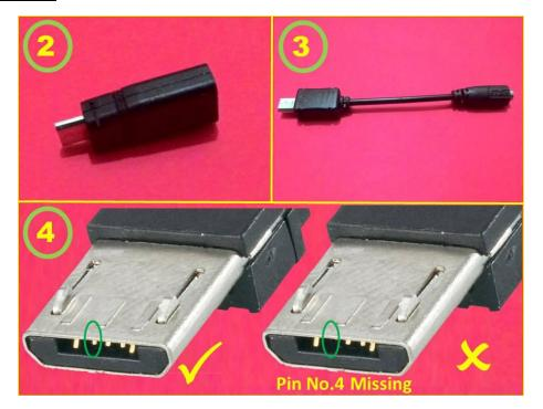
Buy a Micro USB Pin or Buy a charger adapter which cost Rs.10/-Second one may be useful to house the resistor in it. There are two type of adapters are available in the market as shown in Fig. (2) & (3). Both are fine. The problem is number of Pins. Check the number of Pins before buy. Because 4<sup>th</sup> Pin will not be available in some of the charger adapters which is not useful for us. Compare them in Fig. (4). Select adapter which has 5 Pins.
