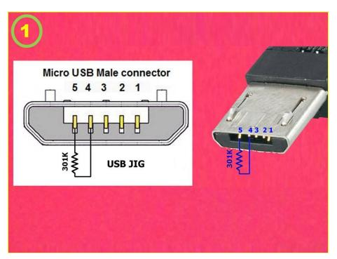
Connecting 301K resistor between Pin No. of 4 and 5 is the USB JIG which force your mobile to boot in Downloading Mode. The schematic shown in Fig (1).
