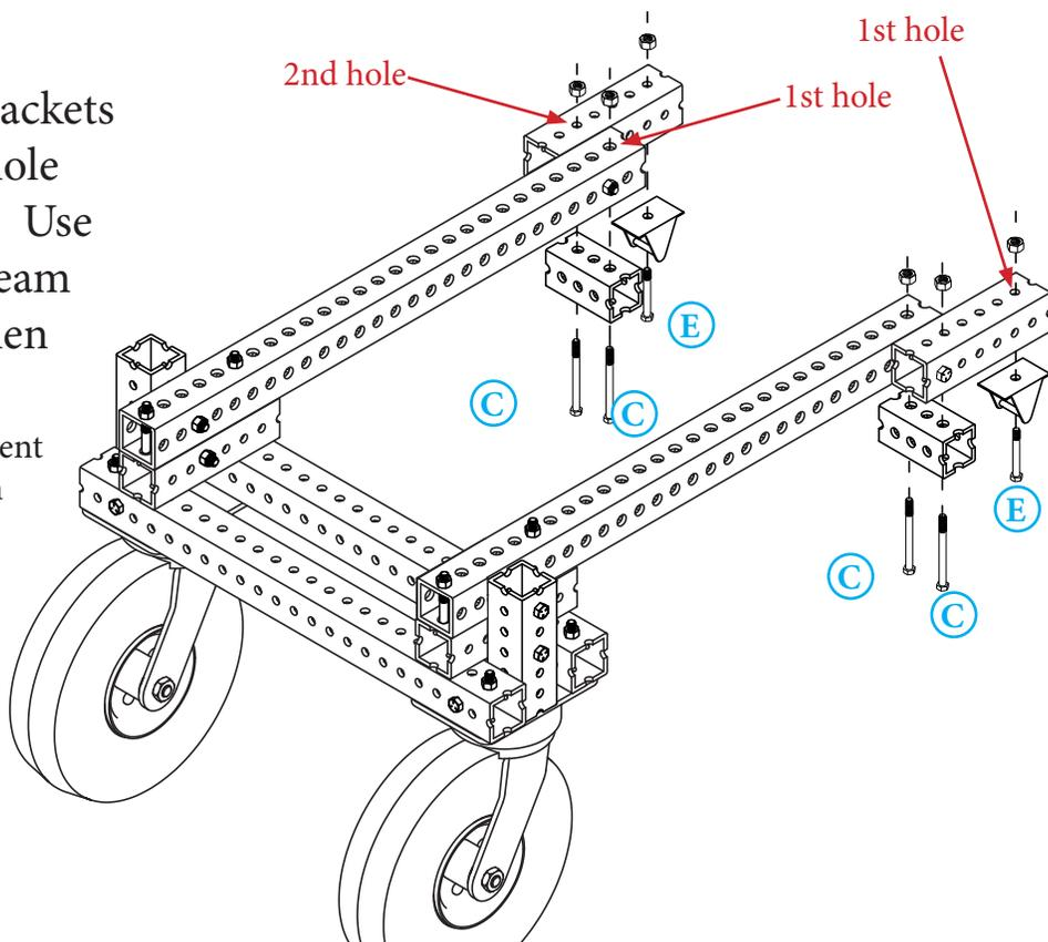
**3** Line the caster assembly and motor assembly together.
