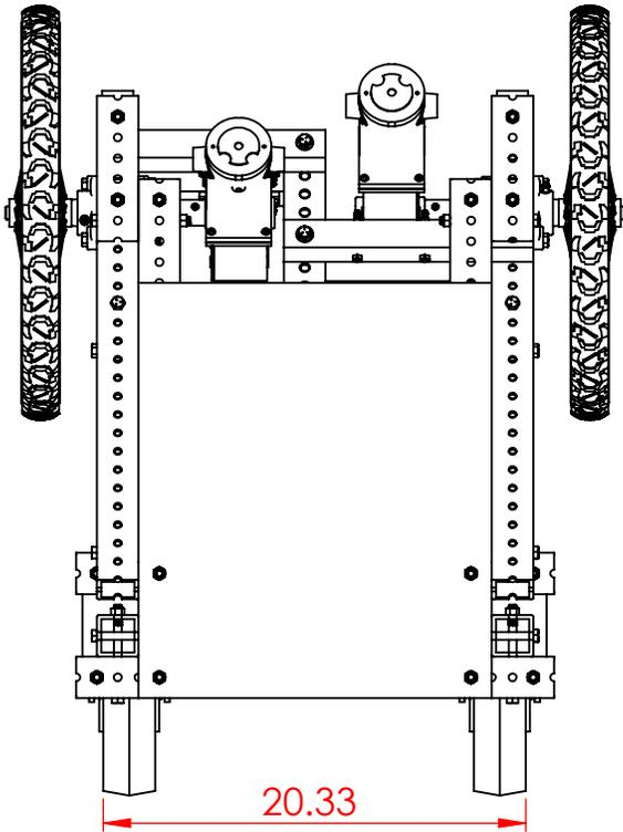
**NOTE:** Although the chair's dimensions (length of ~40" by width of ~30") are within ADA standards, we've determined the width is a large by about 3" to 4". This is addressed in section 5.0 on page 28.
