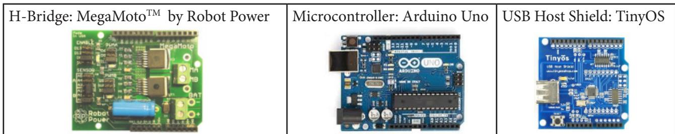
In our prototype we used an Arduino microcontroller in combinations with a MegaMoto™ H-bridge. To incorporate USB devices such as a joystick, we also used a USB host shield. These three boards are designed to stack on top of one another. The configuration of these boards is shown in the block diagram.
