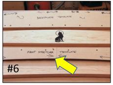
Marking the Positions of the Mortises for the Front Stretcher
