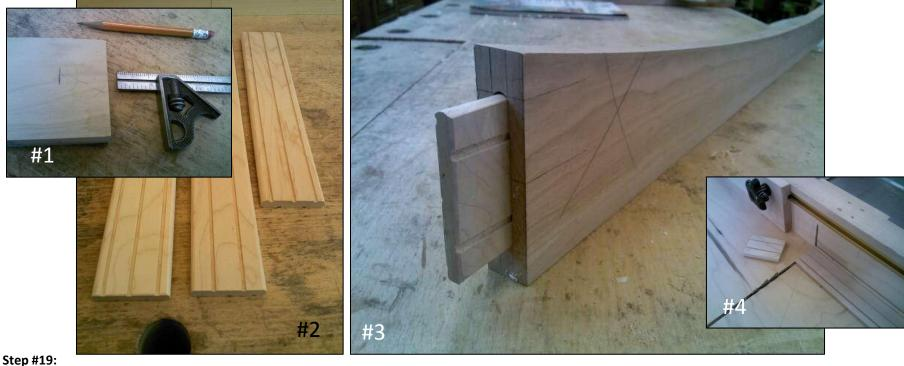
Mill several pieces of hard maple to 3/8" thick for the loose tenons as shown in photo #2. The width and length is dependent on the mortises they fit. Cut a series of 1/16<sup>th</sup> deep grooves along the length on both sides to allow for glue squeeze out. Photo #2 displays the loose tenon stock before they are cut to length.
