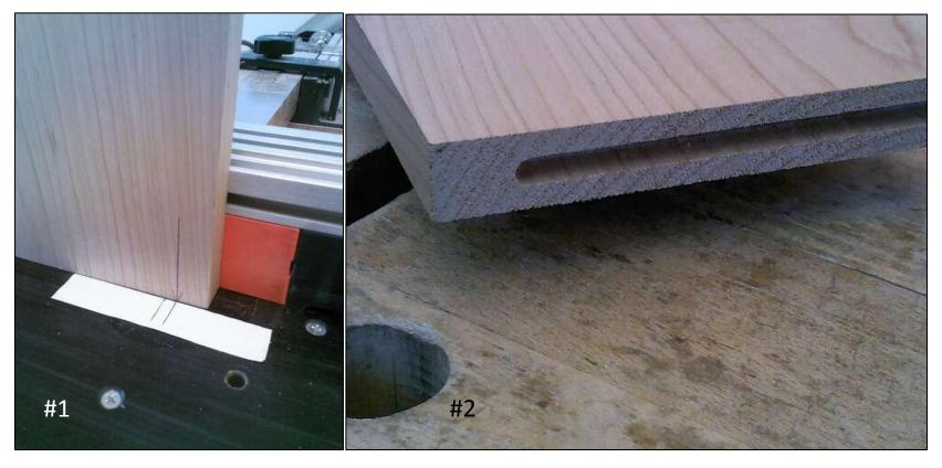
**Step #23:**The vertical dividers need to be sized to fit tightly between the horizontal dividers.
