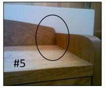
**NOTE:** The backsplash extends above the sides (photo #5) so the mortise on the backsplash has to be positioned accordingly.
