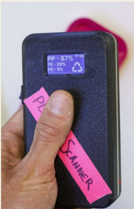
DIY Version of the Plastic Scanner Visual model from thesis Jerry
