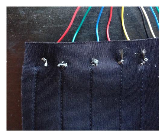
5. To test your switches, you can use the same link as the hookup guide for the capacitive sensor, and download the code that will read and sense which sensor is being touched. Hook up your micro controller to the computer and upload the code. Making sure your sensors are not touching, open your serial monitor and touch a conductive trace - it should detect your touch!
