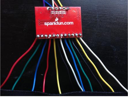
4. Hand sew the ends of the conductive thread onto the corresponding loop of the wires connected to the sensor board. Make sure to make several loops to ensure a strong connection. Trim the leftover thread to make sure that there are no loose ends touching the other traces.
