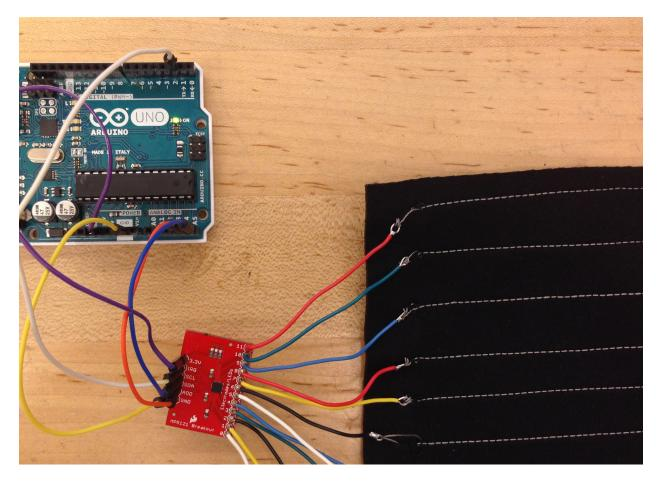
After testing the capacitive touch sensor breakout with various conductive fabric materials, I wanted to create an array of conductive thread traces that could be used to activate the touch sensor instead. This instructable will demonstrate how to connect conductive thread to a capacitive touch sensor, to make switches out of conductive thread.
