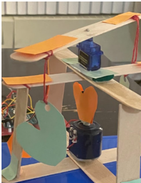
Figure 9: Motor with the stimuli attached, with the motor sitting evenly on the bottom cross. The motor shaft is inserted into the bottom hole from figure 6b.
