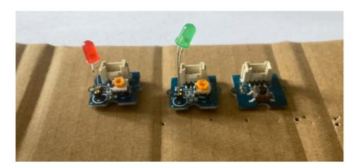
2. Use the Grove cables to connect them to the Grove Shield on the Arduino. Note, for this tutorial, the RED LED is connected to D2. The green LED is connected to D3. And the Button is connected to D4.
