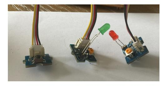
3. Using your screwdriver and some screws or rickets, secure each module to the cardboard.
