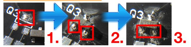
Just like the two leaded components, apply **SOLDERING TIN** to one pad (1) and place the component with a TWEEZER while heating up the pad again. Now generously apply **SOLDERING TIN** to the remaining two or more opposite pads (2), optionally also to the first pad and remove excessive **TIN** one by one (3). **Check the connections using the continuity testing function** of your **MULTIMETER**. Check between leads and from connected leads. Remove unwanted connections with a **SOLDER SUCKER**.
