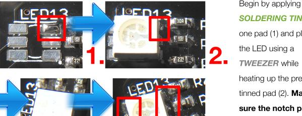
**SOLDERING TIN** to one pad (1) and placing the LED using a TWEEZER while heating up the pretinned pad (2). Make sure the notch points in the opposite direction of the dot printed on the PCB.
