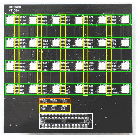
Here you can see the assembled PCB of NerdClock. The colors highlight the group the components belong to.
