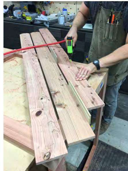
Attaching Redwood Dog Ear Fence Picket to Frame
