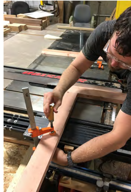
Assembling Framing Members
