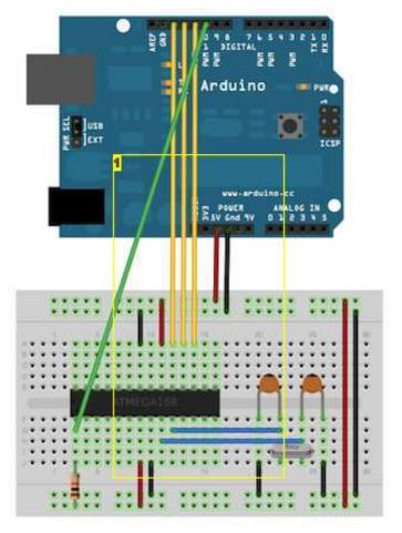
Image Notes 1. Layout for burning bootloader
