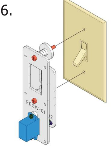
**Note:** Tighten the bottom bolt so the servo switch is held tight but loose enough so the carriage slides freely.
