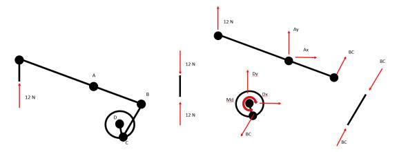
Figure 2: Free-Body-Diagram of Lever Arm Mechanism
