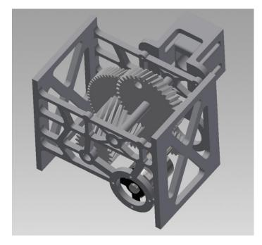
Figure 9: Final Preliminary Gearbox CAD
