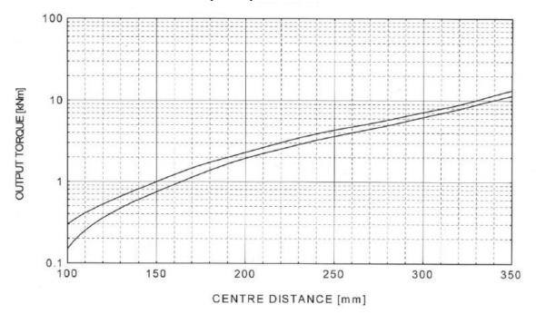
Figure 6: Output Torque vs. Center Distance (borrowed from Technical University of LODZ)
