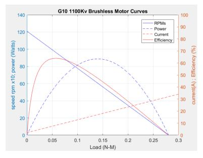
Figure 4: G10 1100Kv Brushless Motor Curves
