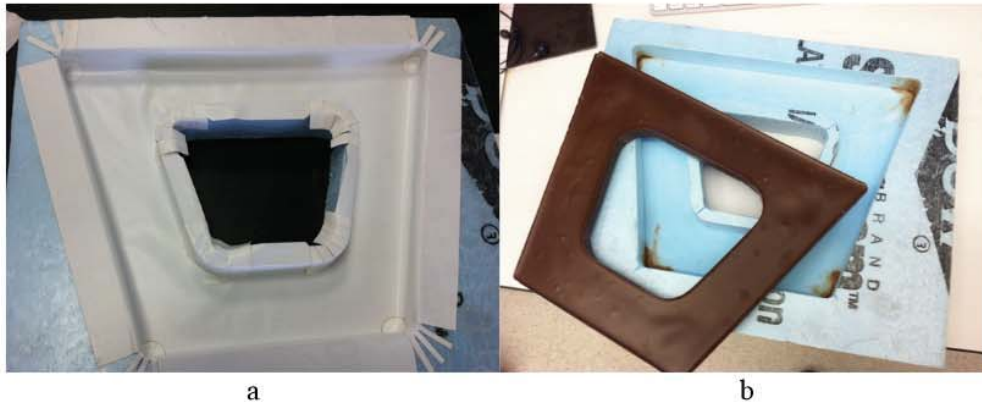
Fig. 9. Large scale molds made from CNC milled Styrofoam. Styrofoam lined with contact paper and the interior wall is flexible for easy release (a). This type of mold is inexpensive and reusable (b).
