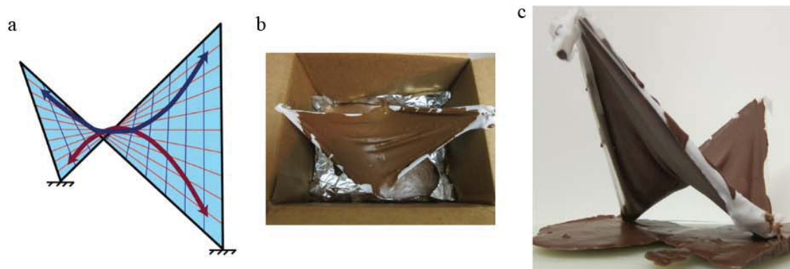
Fig. 4. Structural action in a hyper shape, showing hogging (red) and sagging (blue) behavior (a). Shell formed on pre-stressed fabric formwork before (b) and after (c) being taken down from its supports. (For interpretation of the references to colour in this figure legend, the reader is referred to the web version of this article.)
