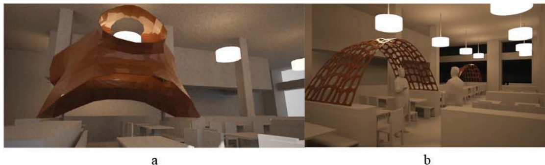
Fig. 12. Volumetric (a) and linear (b) design proposals for a chocolate pavilion that rests on partitions between tables.
