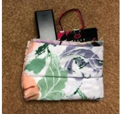
Trim the top edge of the case. Measure the micro:bit. The size is 2"x 1.5". Make the hole by cutting a rectangle shape of the front side of the case. The hole's measurement is 1.8" x 1.25". See figure 3.
