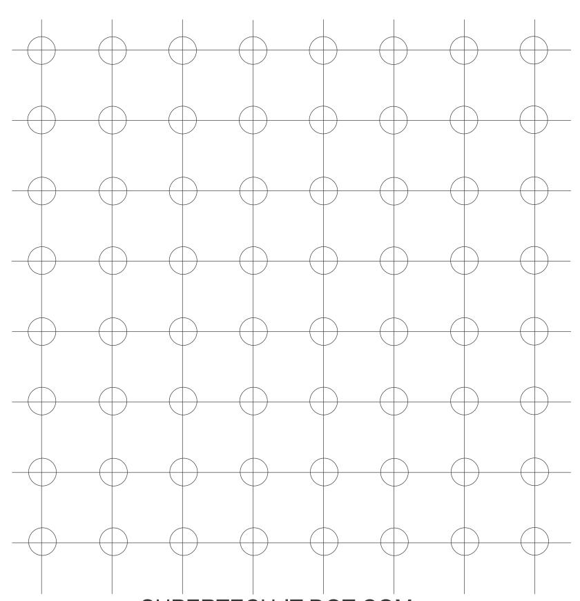
SUPERTECH-IT DOT COM LED Layout Grid for LEDs with 28/29 mm lead length Put holes at grid intersections Ignore circles - not to scale
