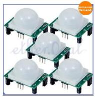
Good sensitivity, large range 7 m. Consumes 60 uA. Unfortunately it is specified to run from 4.5V and runs unreliably from a single LiPo and needs a 1.5V battery in series with power line to boost voltage.
