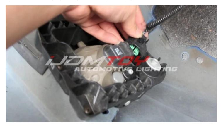
Step 6: After unplugging the harness, feel free to take your whole bumper into a comfortable working environment for optimal concentration. You're going to want to remove Philips head screws with a screwdriver and remove the black bracket securing the fog lamp in.
