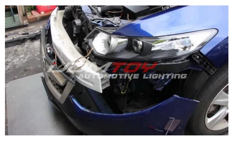
Step 5: Now located the fogs light housing inside the bumper and unplug the harness.
