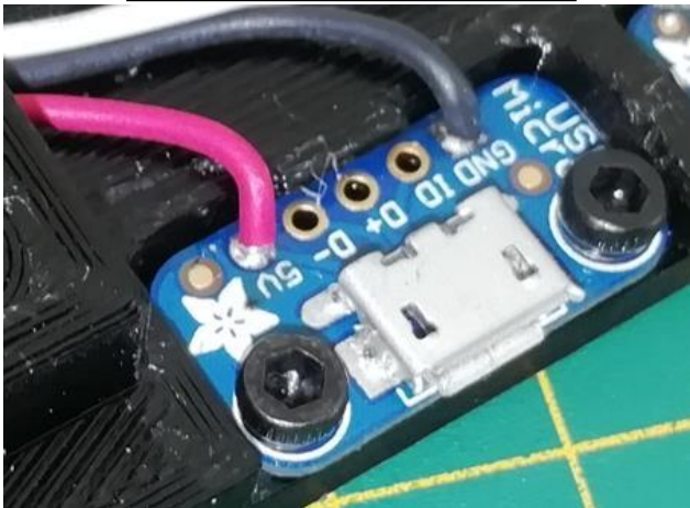
microUSB breakout board: Wire soldering orientation
