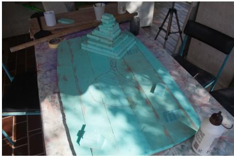
to use for that kind of purpose. You don't have to heat it up for the knife to be glowing red, just keep it over the flame for about 15-20 seconds which will give you about 30 seconds of "work time" with the knife. Wear protective gloves so you don't burn yourself. If you've never done this before, have a few practice cuts on the leftover styro. When it's hot, the knife slices through styro like, you guessed it, a hot knife through butter.
