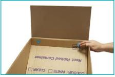
6 Connect the display to the base using Makedo Re-pins and Re-clips. Remember to also secure the other end of the flap to keep the surface at the correct angle.
