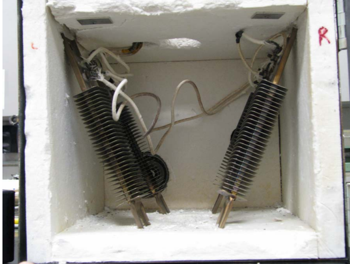
Figure 3.2: Assembled view of oven and heating elements.
