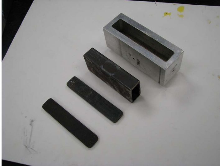
Figure 3.3: Die and load transfer pieces.
