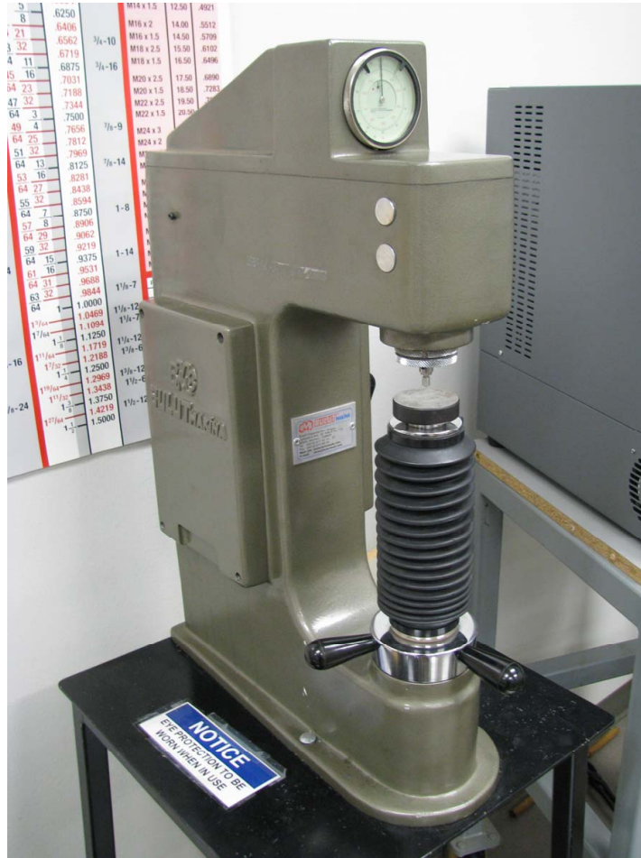
Figure 3.12: Rockwell hardness tester.
