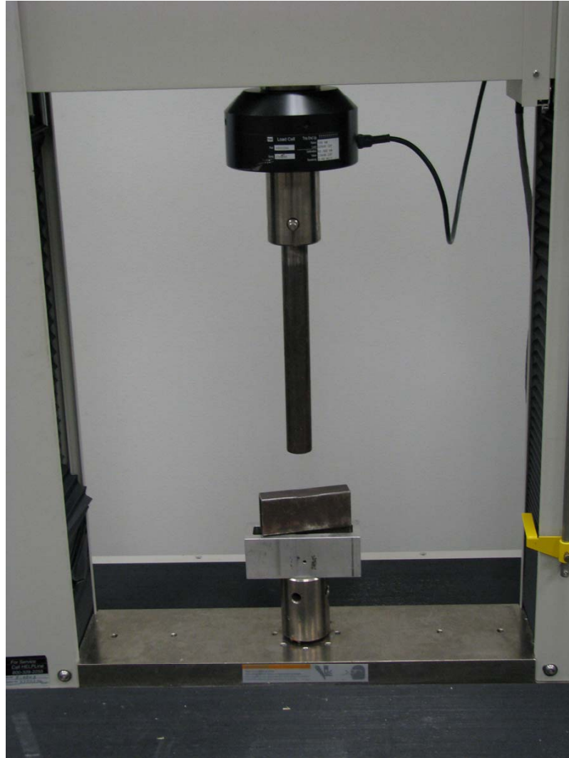
Figure 3.1: Q-Test 100 with punch and die.
