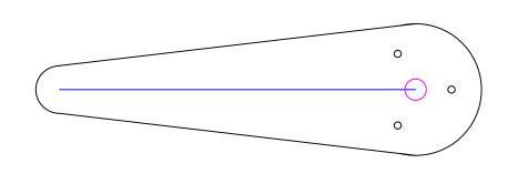
Mount your router onto the jig, and using an oversized cutter, cut a large hole in the jig, to allow for ease of tool change (seen in pink)
