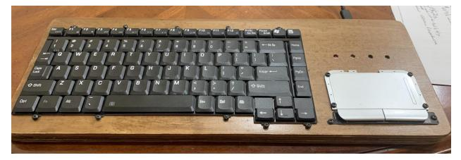
The overall dimensions are 16  $5/8'' \ge 6 1/8'' \ge 11/16''$ . I initially used plastic washers on all the keyboard screws but found they were not needed. Also, washers raise the screw heads up higher, causing them to be felt when pushing the nearby key.
