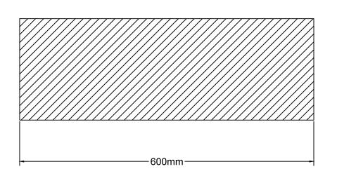
Here is the basic beginning of your circle jig. Hatched; the initial stock that you would use for the jig. I used MDF; 18mm thick, 600mm long, and oversized the width to my router.
