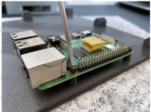
Before screwing the Pi anto the Baseplate, gently screw those M3 screws through the Pi Holes. The Pi comes with M2.5 screws, so we have to widen them to fit M3 screws.
