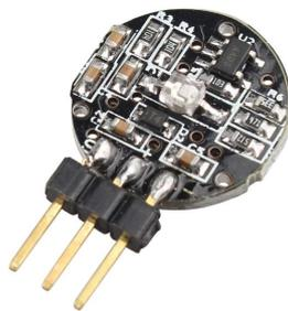
**Instructions:** On the left is the s-pin of the signal output, in the middle is the positive power supply VCC (3.3v ~5V), and on the right is the negative power supply GND.
