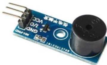
**Instructions:** according to the driving mode is mainly divided into active buzzer and passive buzzer, active buzzer needs dc voltage can drive, passive buzzer needs a specific frequency of vibration signal to drive.The experiment use an active buzzer.
