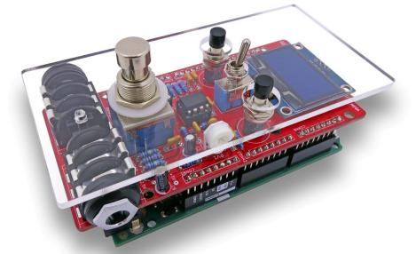
The acrylic cover is kept in placed by the foot-switch nut & plastic washer, simple and practical.
