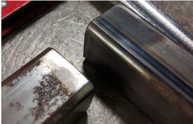
Figure 3: Cleaned Welding Contact Points
