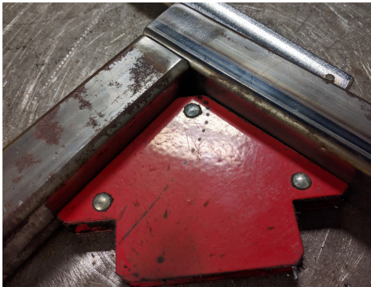
Figure 4: Pipes Fitted to Right Angle
