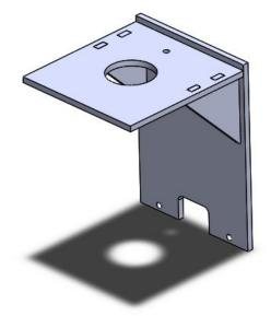
Servo-motor mounting diagram
