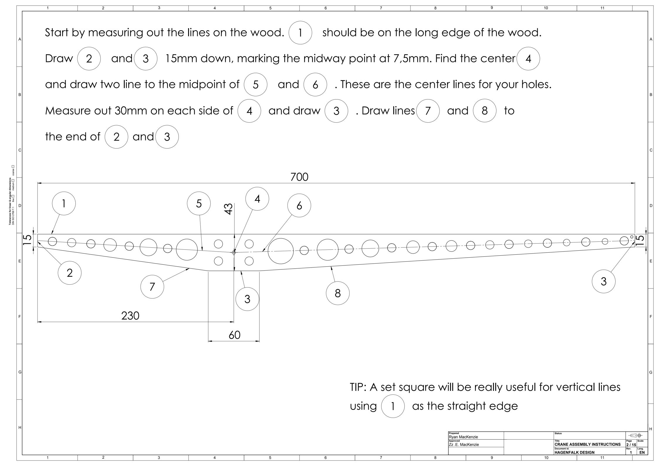
Mark out the locations of the holes. Screw the marked out piece of wood to the unmarked piece, Making sure they line up perfectly. Drill the holes through pieces according to the sizes below. Sand rough or sharp edges and paint all sides, even the inside of the holes. All holes that do not have sizes are 10mm Ryan MacKenzie Zz .E. MacKenzie CRANE ASSEMBLY INSTRUCTIONS
