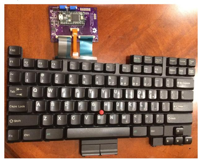
Trackpoint Testing: The trackpoint code "<u>Trackpoint\_380.ino</u>" from the breadboard circuit was loaded into the Teensy and the potentiometers were adjusted to give 1 volt to the X and Y ADC inputs. The trackpoint operation was identical to the breadboard and worked great. Checking the X and Y ADC voltage a day later showed 0.999V and 1.002V. This voltage will be checked over time to see if it changes.
