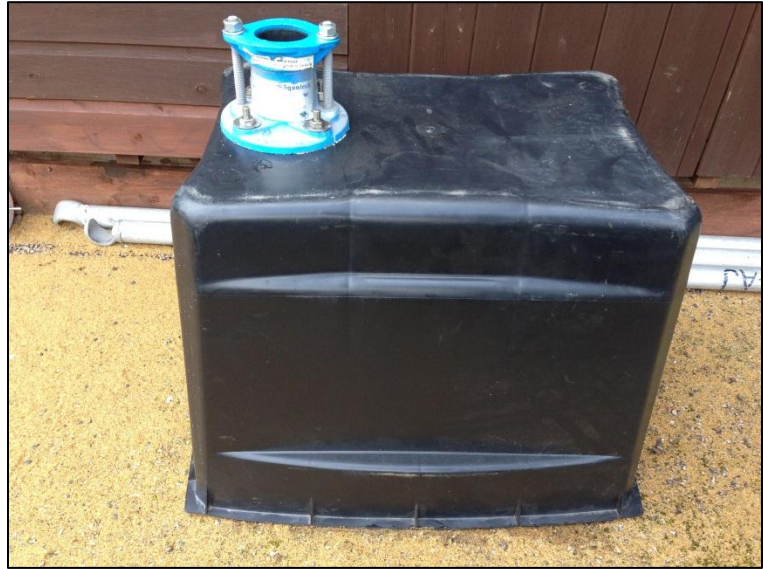
Figure 14: Header Tank (HT) with Flange-Fitting Attached.
