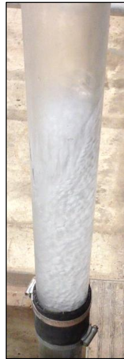
Figure 38: Close-Up of Air in Perspex Pipe. System Off.
