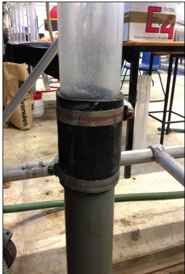
Figure 18: Perspex-Plastic Pipe Connection, Rubber Sleeve & Jubilee Clips
