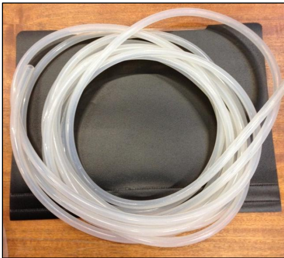
Figure 28: Riser Pipe (RP) Flexible Tubing
