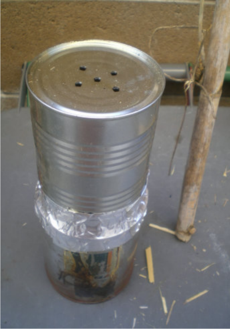
Figure 2 Oven sealed hermetically
