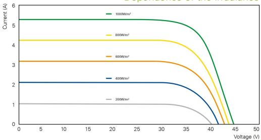
Extracted from BP Solar 175W solar panel specification sheet
