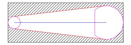
Now to get cutting! using an angle sled on your table saw (i didn't have one at the time so free handed the cut) cut out the shape of your circle jig. (removing the hatched area)
