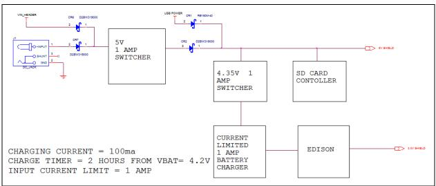
Power from the 5 V switcher is diode-ORed with power from the USB connector. This arrangement allows the Intel<sup>®</sup> Edison kit for Arduino\* to run off external power or USB power. This rail is used to power the shields, the SD card slot, and a 4.35 V switcher. The total current on this rail should be limited to 1 A maximum continuous.
