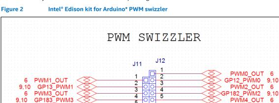
The four PWM sources from the Intel<sup>®</sup> Edison board GP12\_PWM0, GP13\_PWM1, GP182\_PWM2, and GP183\_PWM3 can be configured to drive four of the six Arduino header PWMs. Each Intel<sup>®</sup> Edison board PWM can be jumpered to one of three Arduino PWMs. For example, GP12\_PWM0 can be jumpered to PWM0\_OUT, PWM2\_OUT, or PWM1\_OUT.
