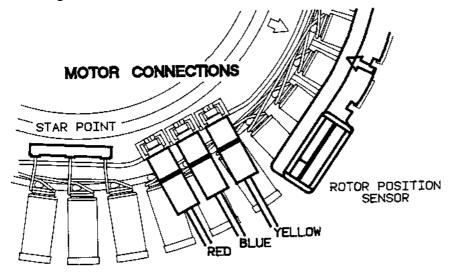
Connect the 3 stator connectors the correct way round, otherwise the motor will not run and give fault code 136. The stator is marked "R B Y".
