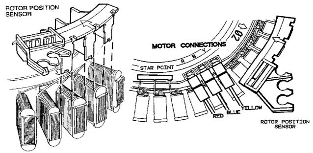
Fault codes 53, 130,131,132,133,134,136 are directly associated with the RPS. Test with a RPS tester. Check the strain relief for the harness. If there is any sign of corrosion replace RPS. If there is an indication of a 'flash over' from the RPS to the stator there will be a black mark on the RPS. The Motor Controller will have blown up.
