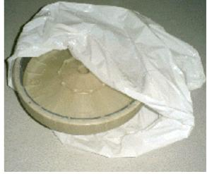
**NB**: When placing the stator on a work bench, ensure the RPS connectors are facing upwards or damage can result. **Do not place the stator inside the rotor.**
