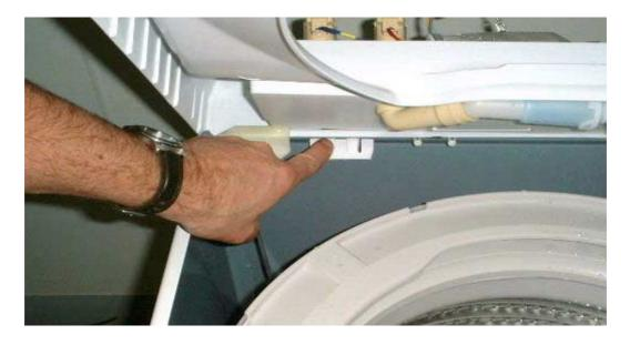
**NB:** The top deck cannot be hinged back without first releasing the rear clips from the cabinet and lifting at the same time.
