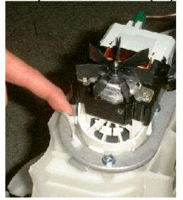
To remove the pump, turn it towards the front of Smartdrive until the locking tab prevents further turning, then release the locking tab by pulling it away from the pump. Continue to turn, the pump will disengage. When refitting the pump, making sure that the bayonet fixture is located correctly. Twist the pump away from the front of Smartdrive until the locking tab clicks into place.
