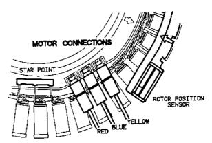
**NB**: The stator should have a slight radial movement of approximately 0.5 - 1mm when correctly tightened and should have maximum axial play (rocking movement) of 0.5mm
