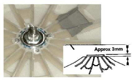
NB: The outer bearing will be proud of the housing by approximately 3mm.
