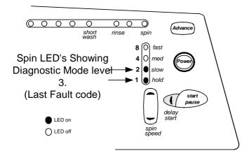
**Note**: The fault code will only be displayed for 8 cycles after the fault has been rectified. If there has been no fault within the last 8 cycles all the wash progress LEDs will be off. In this case it is most unlikely that the Motor Controller will be faulty.
