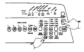
The WASH TEMPERATURE DOWN button turns the Cold Water Valve on. The Cold Water LED will also turn on.
