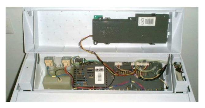
PHASE 5 TOPDECK SHOWING WIRING CONNECTIONS
