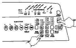
This fault would have occurred within the last 8 cycles. If all the wash progress LEDs are off, there is no fault. Do not change Motor Controller. If there is no fault, (above) and the product will not start check that the lid switch is operating correctly. This may also be done from Diagnostic Mode, see SECTION 8.2.
