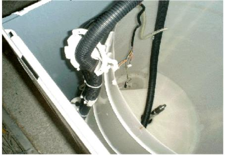
14. Lay the cabinet on its back, on protective material, and slide the outer bowl assembly out, but note that approximately 1 litre of water must be removed from the pump sump before laying the cabinet on its back.
