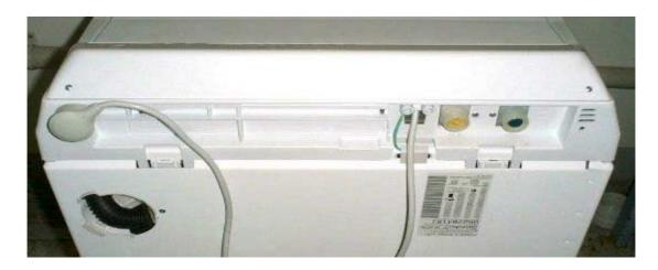
3. Remove the 2 screws from the rear of the top console, disconnect the earth lead. The console can now be raised for access to the Motor Controller Module, Display Module and associated wiring.
