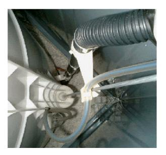
**Drain Hose**. Unclip the drain hose fixture from the lip of the outer bowl and screw into position on the cabinet. Ensure the drain hose grommet is correctly fitted, (photo).
