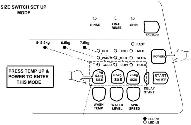
If the size is set incorrectly Smartdrive will have the following settings incorrect: -
