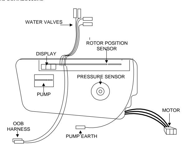
End view of 426418P Motor Controller Module wiring connections.
