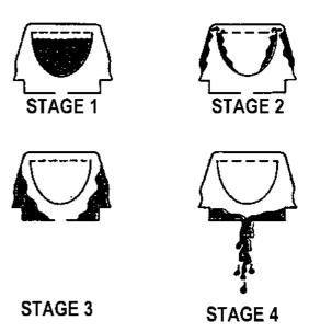
For the Delicate and Permanent Press cycles the fabric softener remains in the dispenser cup throughout the wash and first deep rinse. Smartdrive then spins to release the fabric softener, delivering it down the agitator stem as Smartdrive fills for the final rinse.
