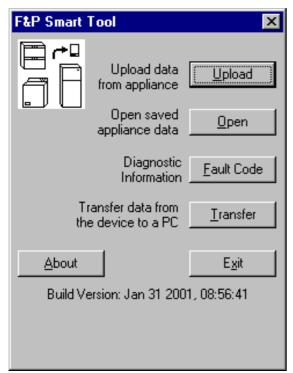
Smarttool is an Application which is run on a PC or a Casiopea Palm-Top. This application may be used with the following Fisher & Paykel products:-
